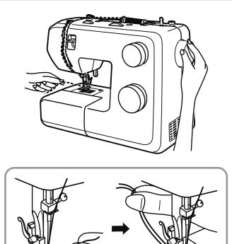
Hold the end of the upper thread with the left hand. Turn the handwheel (21) in the anticlockwise direction until the needle is again raised (a complete revolution).
