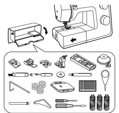
If you want to sew on the arm bed, pull out the snap-in sewing table (7) in the direction of the arrow.
