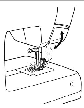
When sewing thick fabrics, the passage of fabrics under the presser foot can be improved by raising the two-step presser foot lifter (17) further (arrow).
