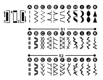
For **straight stitch**, turn the stitch selector dial (6) until it required letter "A" coincides with the mark. You can adjust the needle position from left to central by turning the stitch width dial.
