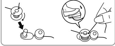
Place the spool (n) on the spool pin (15) and hold it in place with a spool pin cap (s). - Small spool pin cap for thin threads
